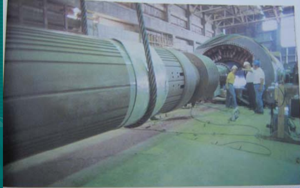
Stator generator rotor being installed.
