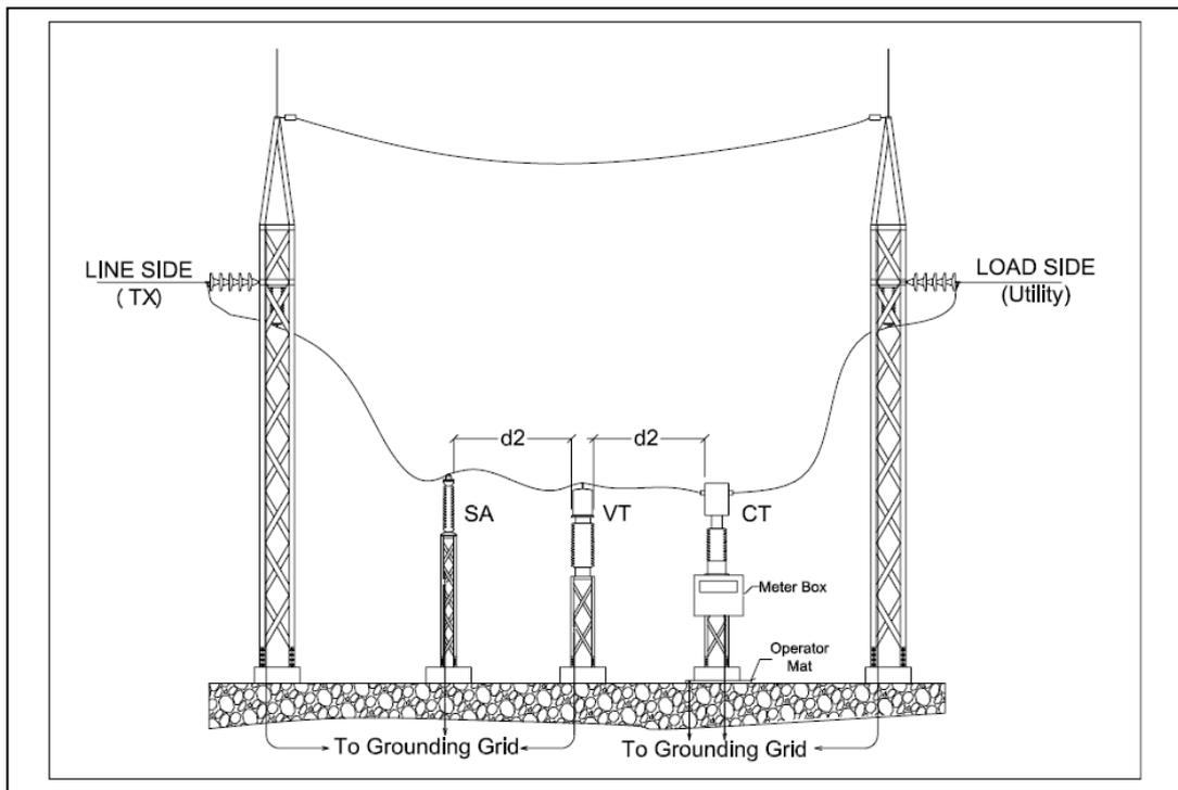
Figure 2(b) - Location/Arrangement of Instrument Transformers
