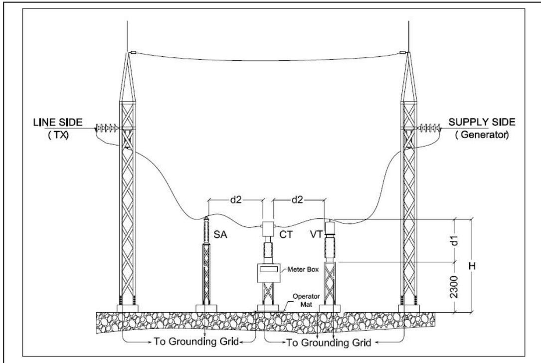
Figure 2(a) - Location/Arrangement of Instrument Transformers (Generator)
