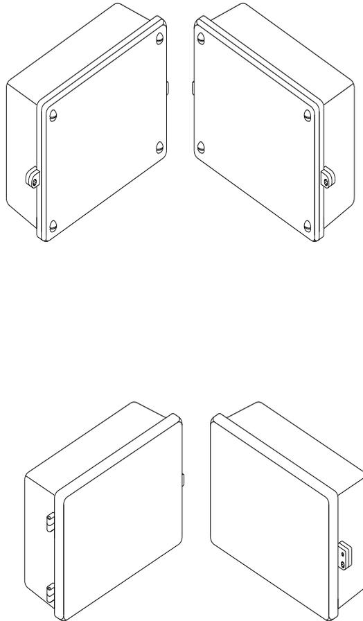
Figure 1 – CT/VT Secondary Terminal Box
