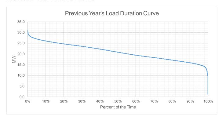
Based on the Load Duration Curve, the minimum load is 10 MW and the maximum load is 32 MW for the last historical year.
