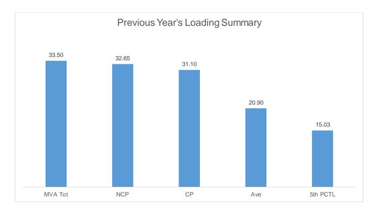
The Non-coincident Peak Demand is 32.5 MW, which is around 97% of the total substation capacity of 33.5 MVA at a power factor of 97.7%. The load factor or the ratio between the Average Load of 20.9 MW and the Non-coincident Peak Demand is 64.4% of. A safe estimate of the true minimum load is the fifth percentile load of 15.03 MW which is 46% of the Non-coincident Peak Demand.
