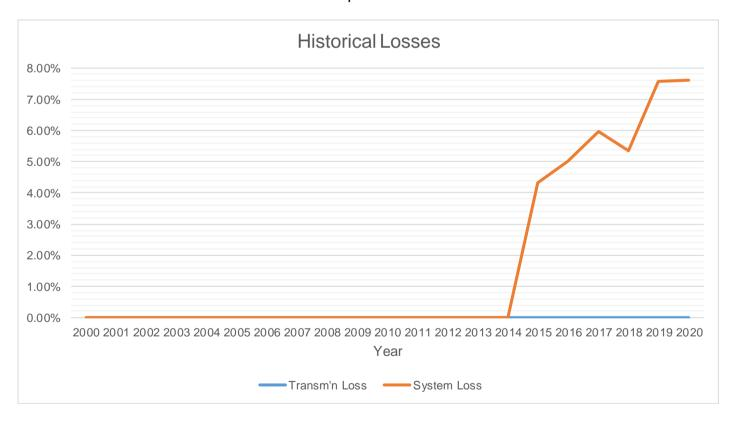
Historically, Transmission Loss is at 0% while System Loss ranged from 4.34% to 7.61%. No Transmission Loss. System Loss peaked at 7.61% on year 2020 because of increasing energy consumption.
