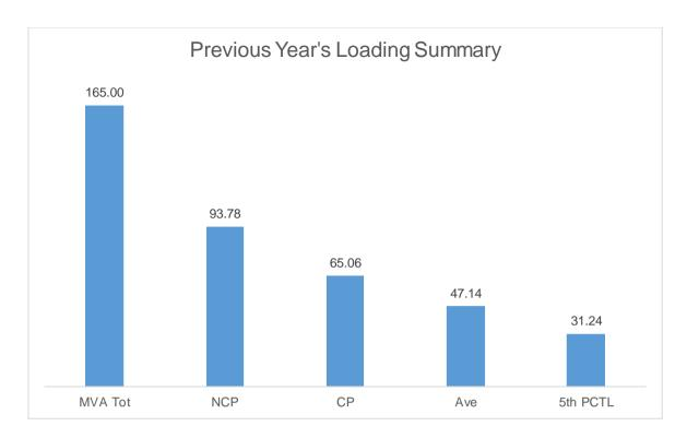
The Non-Coincident Peak Demand is 93.78 MW, which is around 56.83% of the total substation capacity of 165 MVA at a power factor of 92.8%. The load factor or the ratio between the Average Load of 47.14 MW and the Non-coincident Peak Demand is 50.3%. A safe estimate of the true minimum load is the fifth percentile load of 31.24 MW which is 33.31% of the Non-coincident Peak Demand.
