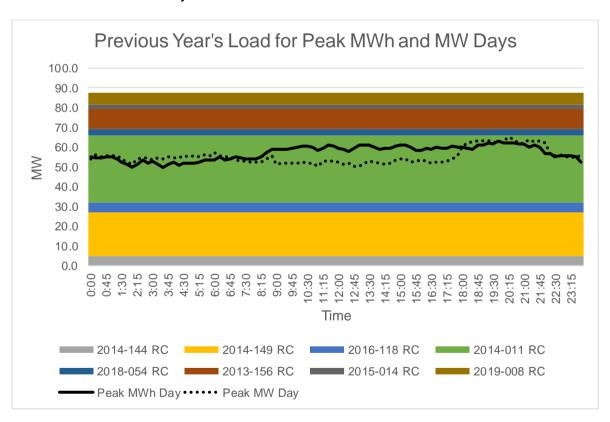
Peak MW occurred on interval 19-21. Peak daily MWh occurred on the same time due to high consumption of residential customers at this interval. As shown in the Load Curves, the available supply is higher than the Peak Demand.
