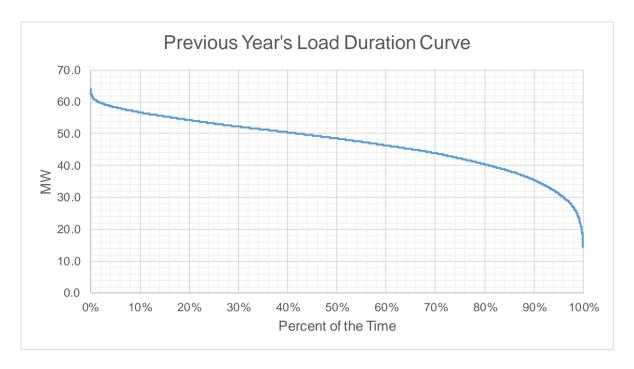
Based on the Load Duration Curve, the minimum load is 14.45 MW and the maximum load is 65.06 MW for the last historical year.
