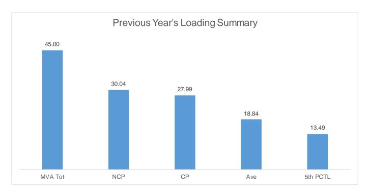
The Non-coincident Peak Demand is 30.04 MW, which is around 68.98% of the total substation capacity of 45 MVA at a power factor of 96.78%. The load factor or the ratio between the Average Load of 18.84 MW and the Non-coincident Peak Demand is 62.72%. A safe estimate of the true minimum load is the fifth percentile load of 13.49 MW which is 44.91% of the Non-coincident Peak Demand.
