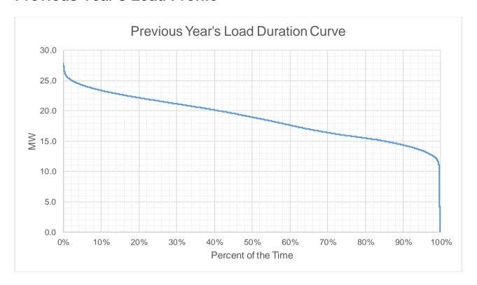
Based on the Load Duration Curve, the minimum load is 12.75 MW and the maximum load is 27.99 MW for the last historical year.
