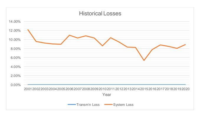
One of the biggest challenges in 2020 in the midst of pandemic was the lowering of ERC SL cap (feeder level) from 6.5% in 2019 to 6.0% in 2020. Cotabato Light hit 8.24% feeder level loss as of December 2020 wherein the cost of excess from the SL cap will be absorbed by the company. CLPC has loss reduction programs which includes CAPEX projects and drastic campaigns to reduce its feeder loss to 5.5% by 2021.
