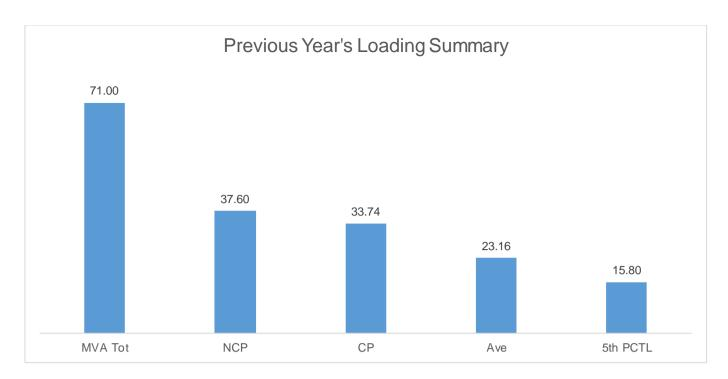
The Non-Coincident Peak Demand is 37.6 MW, which is around 52.42% of the total substation capacity of 70 MVA. The load factor or the ratio between the Average Load of 23.16 MW and the Non-Coincident Peak Demand is 61.60% of 37.60 MW. A safe estimate of the true minimum load is the fifth percentile load of 15.80 MW which is 42.02% of the Non-Coincident Peak Demand.
