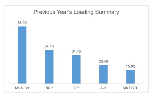
The Non-coincident Peak Demand is 37.16 MW, which is around 58.98% of the total substation capacity of 63 MVA. The load factor or the ratio between the Average Load of 20.46 MW and the Non-coincident Peak Demand is 55.1% of. A safe estimate of the true minimum load is the fifth percentile load of 15.02 MW which is 40.4% of the Non-coincident Peak Demand.
