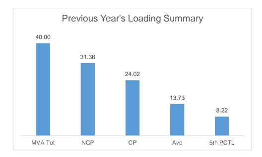
The Non-coincident Peak Demand is 31.36 MW, which is around 78.40% of the total substation capacity of 40 MVA at a power factor of 95%. The load factor or the ratio between the Average Load of 13.73 MW and the Non-coincident Peak Demand is 43.78% of. A safe estimate of the true minimum load is the fifth percentile load of 8.22 MW which is 26.21% of the Non-coincident Peak Demand.
