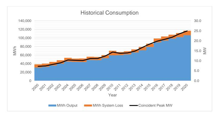
MWh Output increased from year 2019 to year 2020 at a rate of 4.71%, while MWh System Loss increased at a rate of 4.38% within the same period in proportion with the increase of MWh Output.
