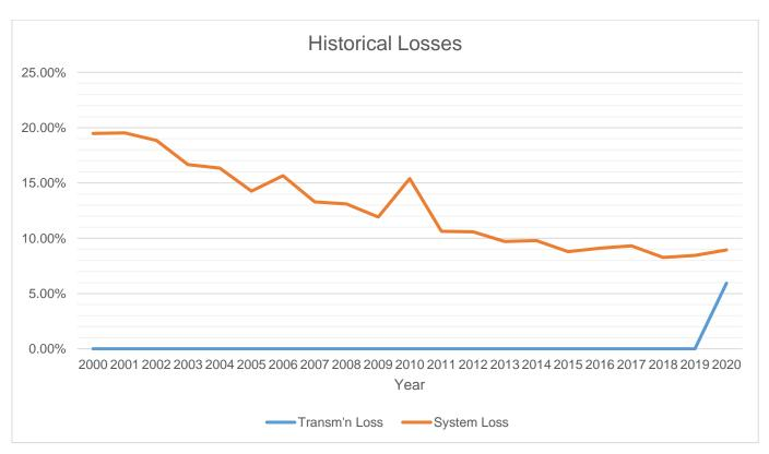
Historically, System Loss on the year 2000 decreased from 19.48% to 8.93% on the year 2020. System Loss peaked at 19.48% on year 2000 because of the design of the system that time. The decrease on system loss was due to the construction of new substations, line rehabilitation, pole metering activities and assuring the quality of kilowatt-hour meters being installed to customers.
