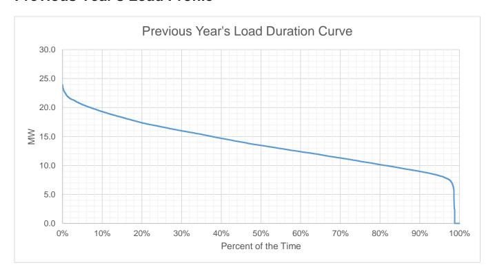
Based on the Load Duration Curve, the minimum load is 9.79MW and the maximum load is 24.02 MW for the last historical year(coincidental).
