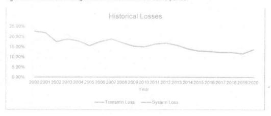
Historically, System Loss ranged from 11.64% to 22.72%. System Loss peaked at 21.98% and 22.72% on years 2001 and 2000, respectively, because of minimal system loss reduction activities that were implemented previously. Additionally, exposure to Typhoon Reming in 2000 and Typhoon Emong in 2009 have also contributed to the increase in system loss.
