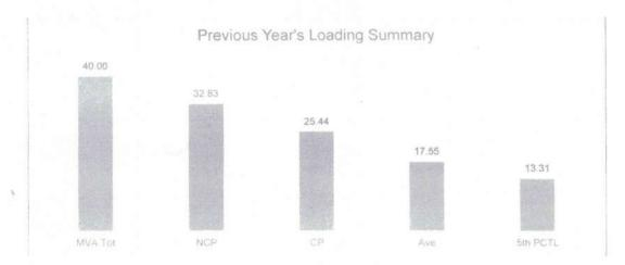
The Non-coincident Peak Demand is 32.83 MW, which is around 82.08% of the total substation capacity of 40.00 MVA at a power factor of 98 %. The load factor or the ratio between the Average Load of 17.55 MW and the Non-coincident Peak Demand is 53.46%. A safe estimate of the true minimum load is the fifth percentile load of 13.31 MW which is 40.54% of the Non-coincident Peak Demand.
