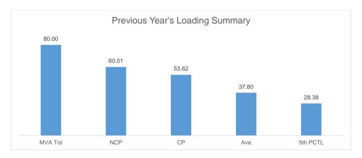
The Non-coincident Peak Demand is 60.51 MW, which is around 75.64% of the total substation capacity of 80 MVA at a power factor of 0.978. The load factor or the ratio between the Average Load of 37.80 MW and the Non-coincident Peak Demand is 62.47%. A safe estimate of the true minimum load is the fifth percentile load of 28.38 MW which is 46.90% of the Non-coincident Peak Demand.
