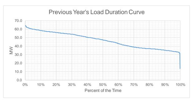
Based on the Load Duration Curve, the minimum load is approximately 13.4 MW and the maximum load is approximately 68 MW for the last historical year.
