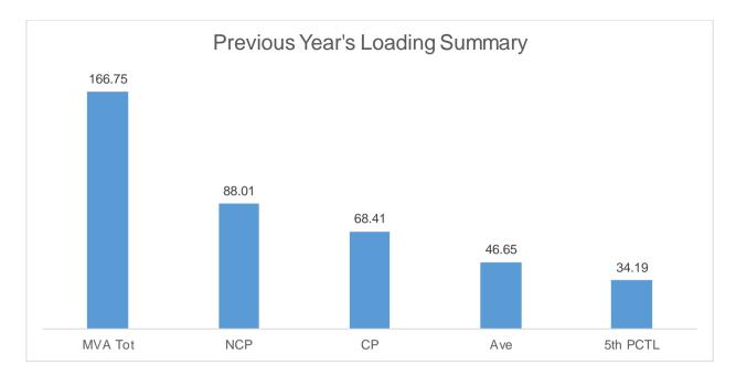
The Non-coincident Peak Demand is 88.01 MW, which is around 53% of the total substation capacity of MVA at a power factor of 0.98. The load factor or the ratio between the Average Load of 46.65 MW and the Non-coincident Peak Demand is 63%. A safe estimate of the true minimum load is the fifth percentile load of 34.19 MW which is 39% of the Non-coincident Peak Demand.
