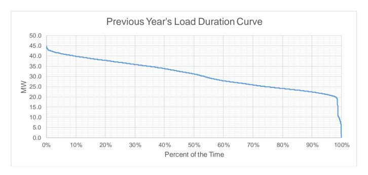
Based on the Load Duration Curve, the minimum load is around 22.5 MW. And the maximum load is 44.756 MW for the last historical year.
