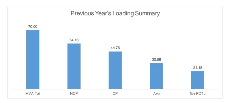
The Non-coincident Peak Demand is 54.16 MW, which is around 77% of the total substation capacity of 70 MVA at a power factor of 0.9. The load factor or the ratio between the Average Load of 30.86 MW and the Non-coincident Peak Demand is 57% of. A safe estimate of the true minimum load is the fifth percentile load of 21.18 MW which is 39% of the Non-coincident Peak Demand.
