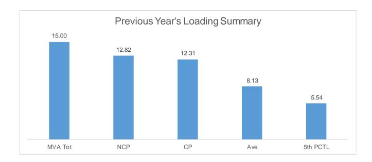
The Non-coincident Peak Demand is 12.82 MW, which is around 75.97% of the total substation capacity of 15 MVA at a power factor of 95.3%. The load factor or the ratio between the Average Load of 8.13 MW and the Non-coincident Peak Demand is 63.416% of. A safe estimate of the true minimum load is the fifth percentile load of 5.54 MW which is 43.214% of the Non-coincident Peak Demand.
