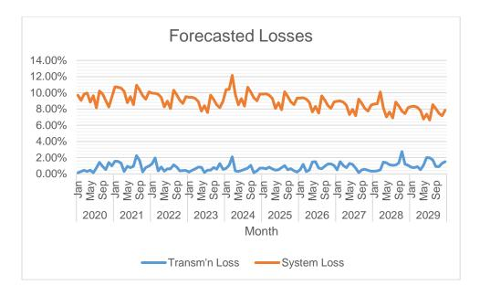
Transmission Loss is expected to range from 2.75 % to 0.12 % while System Loss is expected to range from 10.24 % to 7.72 %
