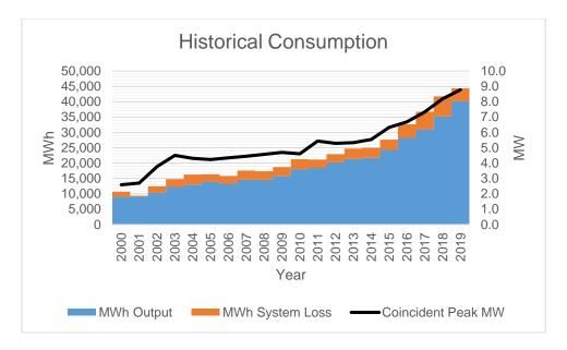
MWh Output increased from year 2018 to year 2019 at a rate of 13.10 %, while MWh System Loss decreased from 15.60% in year 2018 to 9.43% in year 2019 due to new to substation.
