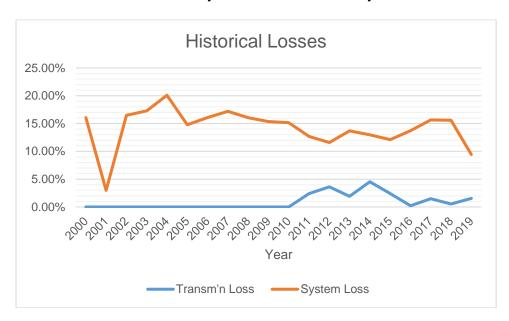
Historically, the overall Transmission Loss ranged from 0.53% to 4.53% while the overall System Loss ranged from 15.65% to 9.43%.
