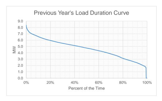
Based on the Load Duration Curve, the minimum load is 2.14 MW and the maximum load is 9 MW for the last historical year.
