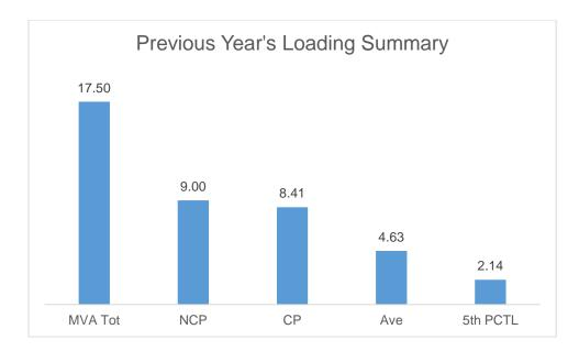
The Non-coincident Peak Demand is 9 MW, which is around 29% of the total substation capacity of 23 MVA at a power factor of 97.52%. A safe estimate of the true minimum load is the fifth percentile load of 2.14 MW which is 23% of the Non-coincident Peak Demand.
