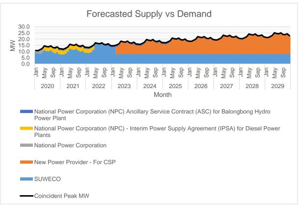
At present, there is no deficit in power supply in Catanduanes because of Amendment 1 (5 MW) and 2 (6.6 MW) of the Electricity Supply Agreement (ESA) between FICELCO and Sunwest Water Electricity Corporation, Inc (SUWECO) as backed-up to the undelivered/not completed Hitoma 2 and Capipian Hydro Power Plant under the original ESA. As stipulated in these amendments, the backed-up diesel-fueled generators will also augment the power deficiency in Catanduanes.
