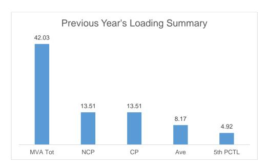
The Non-coincident Peak Demand is <u>13.51 MW</u>, which is around <u>32.14%</u> of the total capacity of 42.03 MVA at a power factor of 85%. The load factor or the ratio between the Average Load of 8.17 MW and the Non-coincident Peak Demand is <u>60.47%</u>. A safe estimate of the true minimum load is the fifth percentile load of 4.92 MW which is 36.42% of the Non-coincident Peak Demand.
