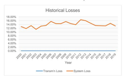
For the past five years, the average system loss is 13.53%. The overall system loss peaked at 16.48% on year 2012 due to ROW clearing problems/issues and embedded power plants at FICELCO's franchise area.
