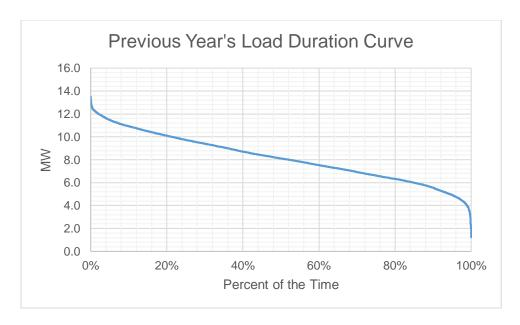
Based on the Load Duration Curve, the maximum load is 13.505 MW for the last historical year
