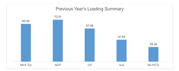
The Non-coincident Peak Demand is 72.31 MW, which is around 139% of the total substation capacity of 65 MVA at a power factor of 0.80. The load factor or the ratio between the Average Load of 37.84 MW and the Non-coincident Peak Demand is 52.33% of. A safe estimate of the true minimum load is the fifth percentile load of 25.2 MW which is 34.85% of the Non-coincident Peak Demand.
