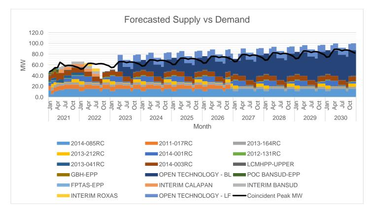
Of the available supply, the largest is 47 MW from the Base Load Open Technology Power Plant. This is followed by 15 MW from DMCI Power Corporation.
