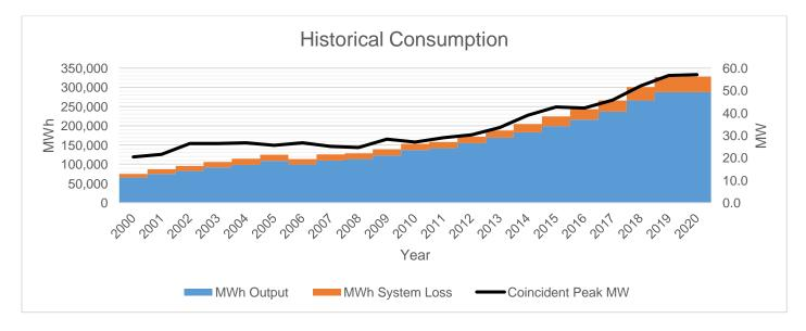
MWh Output decreased from year 2019 to year 2020 at a rate of 8.20%, while MWh System Loss increased at an average rate of 2.08% within the same period. Note that transmission loss are include to the system loss reflected on the table above.
