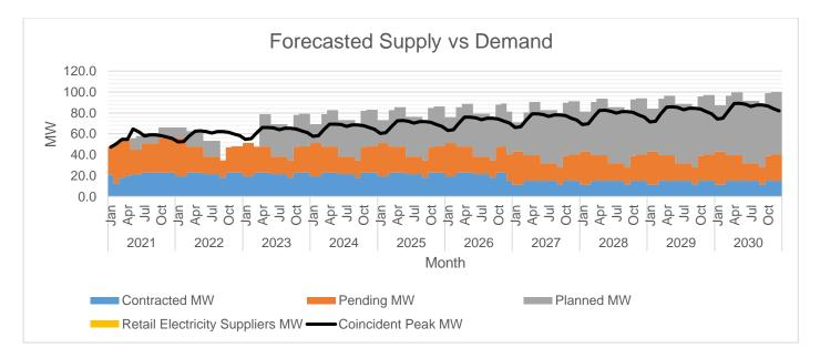
The available supply is generally above the Peak Demand from year 2021 to 2030. This is because of the Planned 60MW new power plant to be installed at Roxas, Calapan and Pinamalayan Oriental Mindoro wherein 47 MW of this supply was base load and 13 MW was mid merit.
