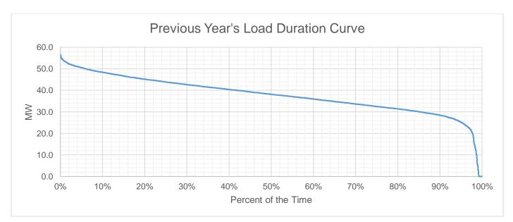
Based on the Load Duration Curve, the minimum load is 0 MW and the maximum load is 57.08 MW for the last historical year. We recorded 0 MW because Oriental Mindoro was hardly hit by typhoon Quinta last October 2020.
